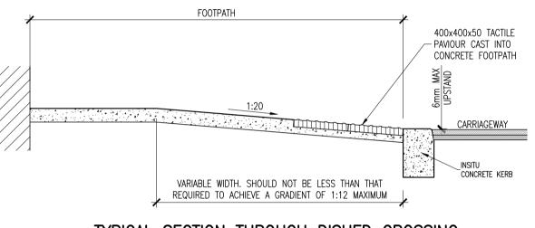
TYPICAL SECTION THROUGH DISHED CROSSING SCALE 1:25
